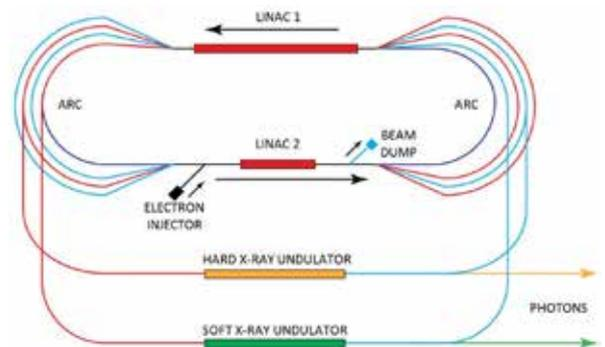
Schematic of a generic recirculating energy recovery accelerator with multiple arcs for different energy beams
