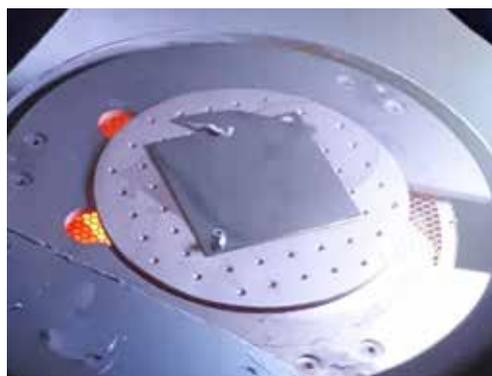
A niobium film deposited on a pre-prepared pure copper substrate
