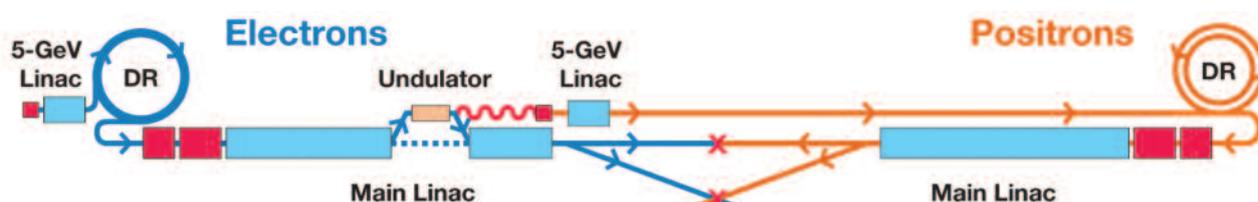
Schematic layout of the International Linear Collider.
