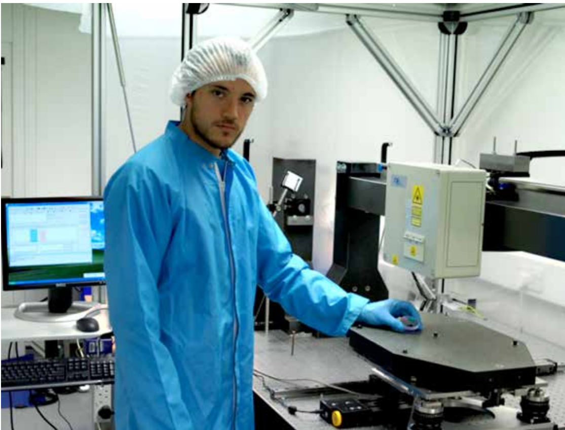
Reuben Santer is seen placing one of the laser mirrors onto the measuring stage of the LTP in the Optics Metrology Laboratory
