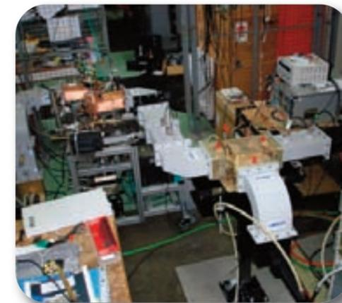
High Power RF coupler undergoing final tests
