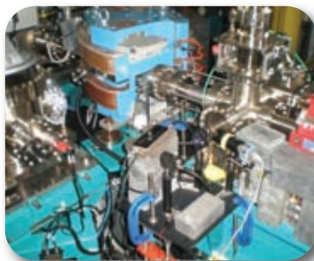
focusing of laser and electron beams & transverse alignment
