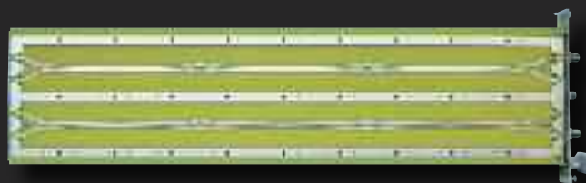
EMMA BPM converter (coupler is open)
