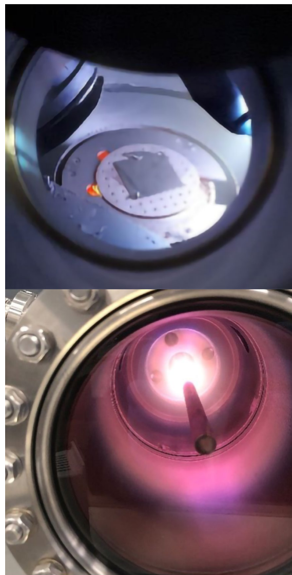
Superconducting thin film deposition facilities in ASTeC's VISTA laboratory for planar surfaces (top) and accelerator cavities(bottom).
