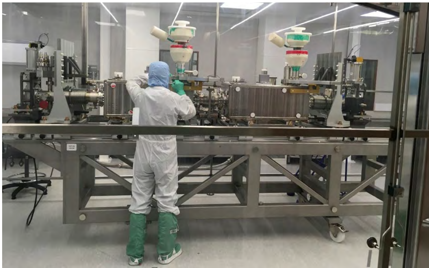
Successfully integrating the Crab Cavity String in the ISO-4 Clean room.
