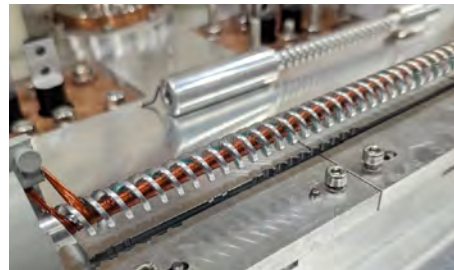
A prototype of the superconducting undulator under construction.
